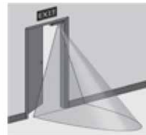
REX shown adjusted for door approach
